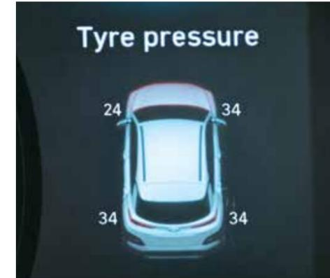
Tyre pressure monitoring system (high line)
