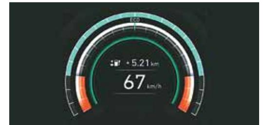
Smart eco pedal guide-encourages fuel efficient driving
