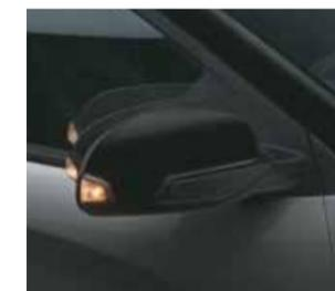
ORVM (heated) with electric adjust and folding
