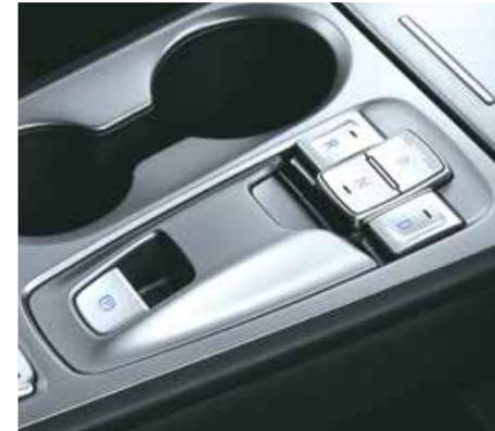
Shift-by-wire automatic transmission and electric parking brake
