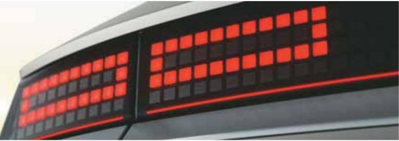
Parametric pixel LED taillamps
