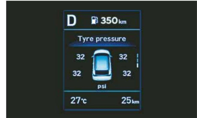
Tyre pressure monitoring system (highline)
