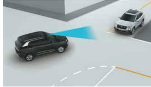
Forward Collision - Avoidance Assist - Junction Turning (FCA-JT)
