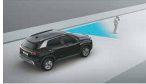
Forward Collision - Avoidance Assist - Pedestrian (FCA-Ped)
