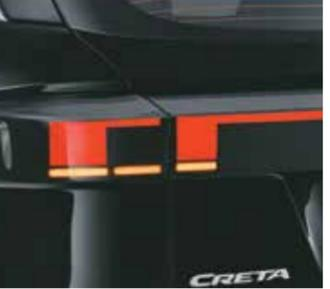
LED rear turn signal with sequential function
