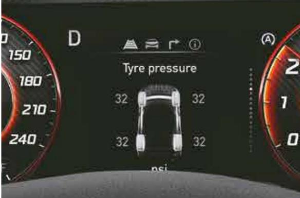
Tyre pressure monitoring system: Highline
